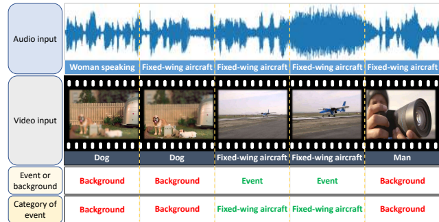
Fig. 1. An example of the audio-visual event localization. The goal of AVE localization is to predict the event label for each segment of a given video sequence. An event that is both audible and visible is regarded as an audio-visual event (“Fixed-wing aircraft” in the third and fourth segments). On the contrary, a segment is not both audible and visible, which is predicted as background. In addition, the asynchronous situation makes the AVE localization more challenging, for example, the sound of the fixed-wing aircraft is heard in the second segment, while the appearance of fixed-wing aircraft is seen in the third and fourth segments.
