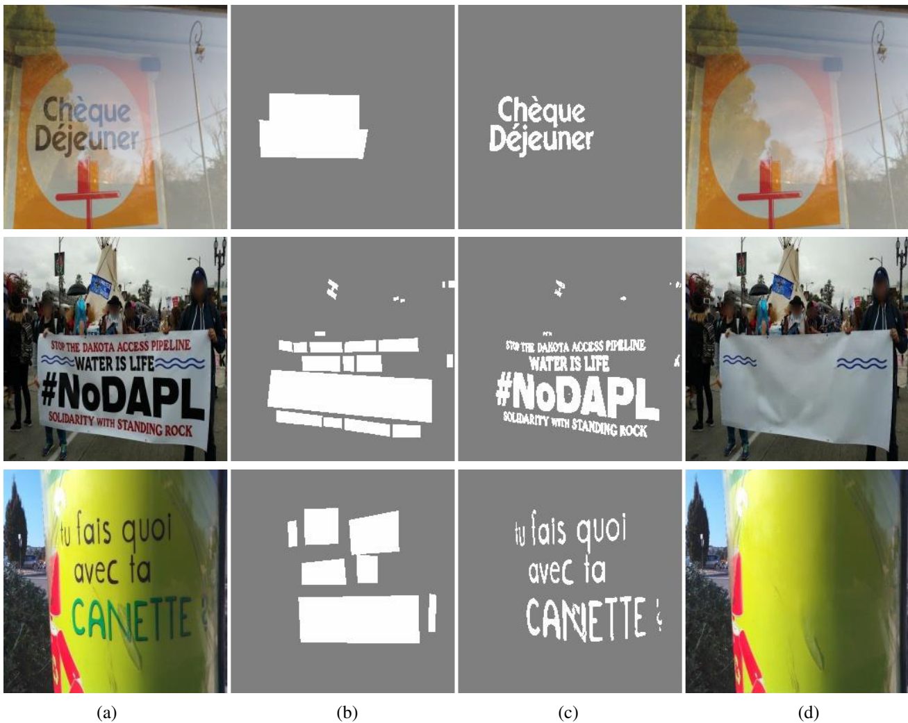
Fig. 1. Sampled results of the proposed scene text removal method. From left to right: (a) input image, (b) the region mask, (c) text stroke mask obtained by our TSDNet, and (d) the final result. Each row shows a representative result of commonly appeared scenarios.
