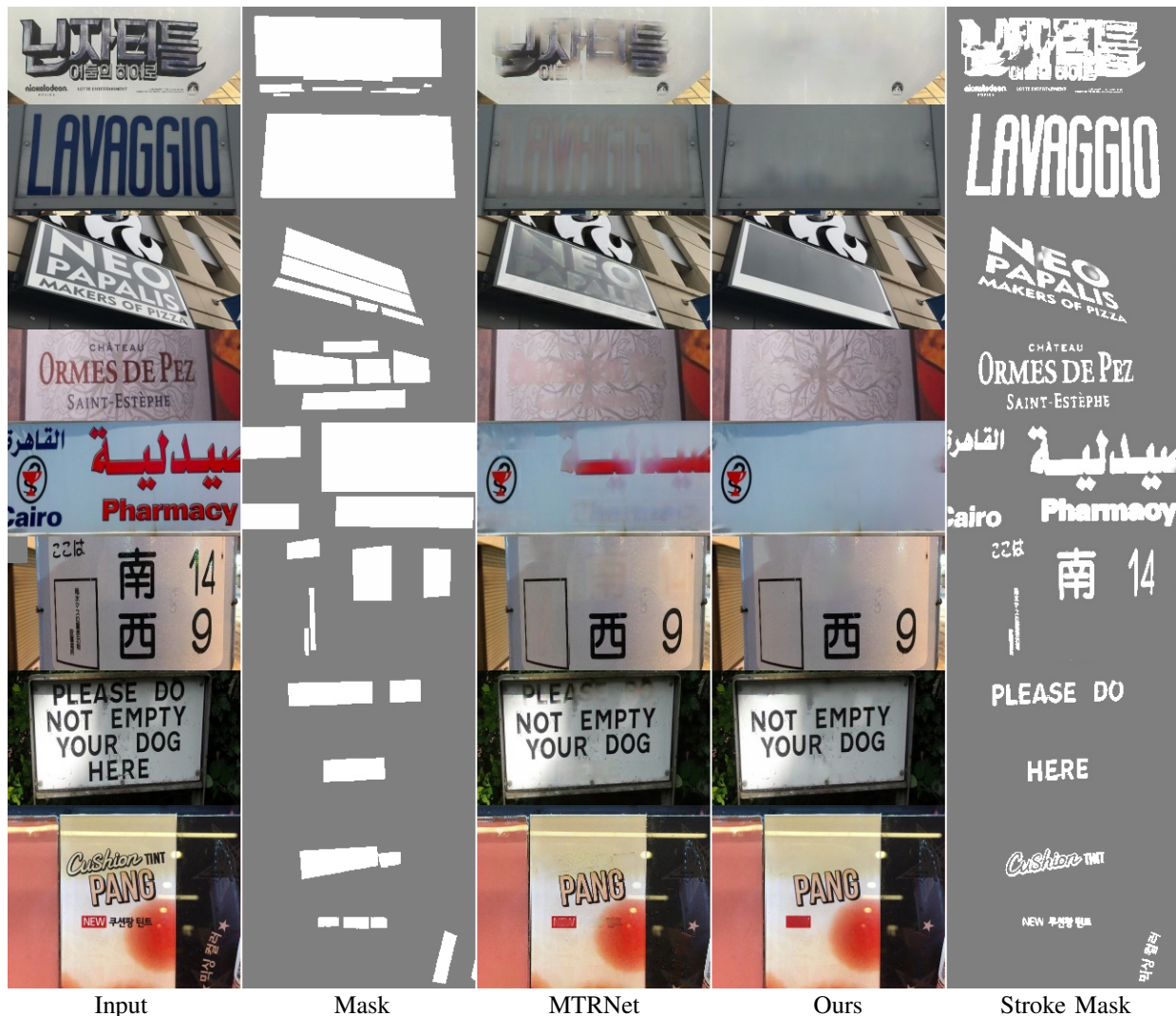
Fig. 8. Results of multi-lingual text removal and selective text removal (the last three rows). From left to right: original image, input mask, MTRNet output, our output, and detected stroke mask of our method. Both models are trained on our dataset.
