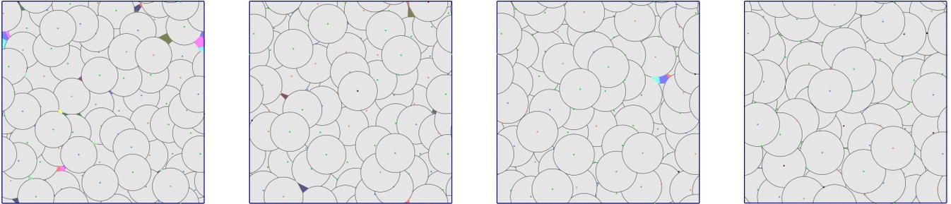
**Figure 1:** The work flow of our method. From left to right: initial point set, the result after 50 iterations, the result after 100 iterations, and the final result. By iteratively adjusting the position of points and the sampling radius, the gap regions (colorized polygons) become smaller and smaller. Finally, the sampling becomes maximal.
